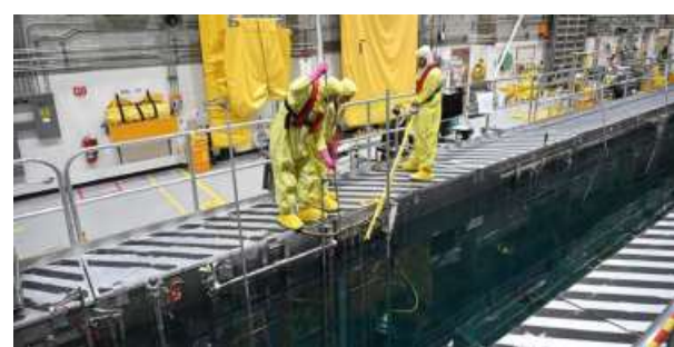
INNOVATIVE TECH. Capsules of ANEEL fuel for accelerated irradiation testing being loaded in the advanced test reactor at Idaho National Laboratory
